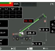
The crane's work is secured by the WIDE MSC670 LMI(Load Moment limiter),delivers the industry's most reliable electronic monitoring system available (HIRSCHMANN as option) .
