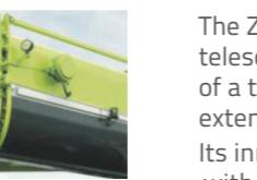
The ZRT850 features a 5-section, U-shaped ,47m telescopic boom.It's telescoping system consists of a two-stage hydraulic cylinder with a rope extension mechanism.
